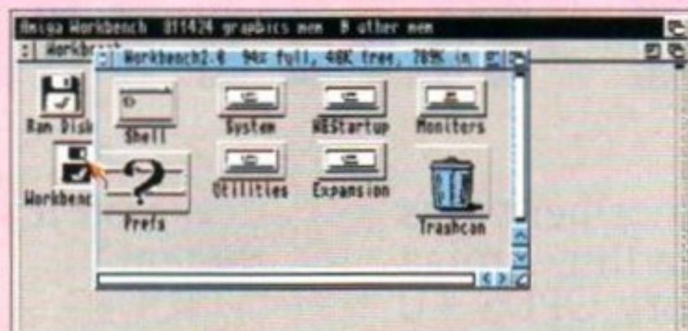
1 Load your Workbench disk. Open the disk, find the icon that says Shell or CLI and double-click on it.
